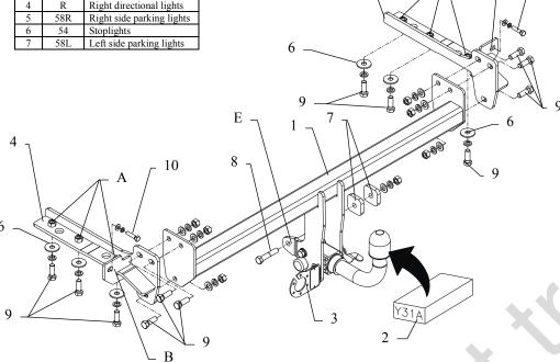
This towbar is designed to assembly in following cars: HONDA FR-V, VAN produced since 02.2005 till 12.2010, catalogue no. Y31A and is prepared to tow trailers max total weight 1500 kg and max vertical load 90 kg.
