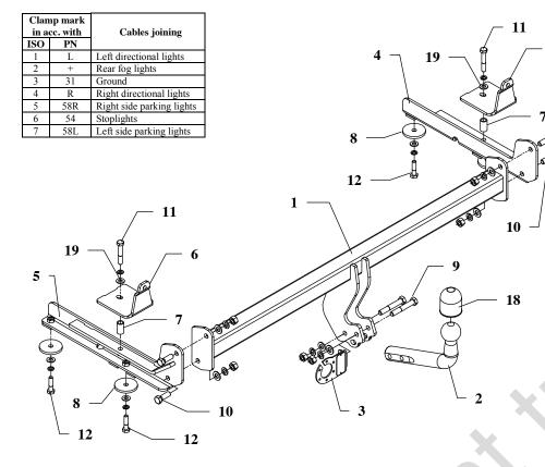
This towing hitch is designed to assembly in following car: **HONDA ACCORD, 4/5 doors (CD7, CD8, CD9),** produced since 03.1993 till 10.1998, catalogue no. **Y22** and is prepared to tow trailers max total weight **1400 kg** and max vertical load **70 kg**.
