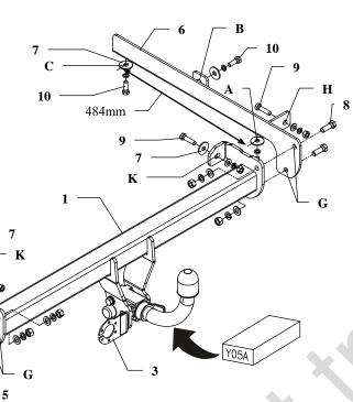
This towing hitch is designed to assembly in following cars: **HONDA CIVIC AERODECK ESTATE**, produced since 1997 till 02.2001, catalogue no. **Y05A** and is prepared to tow trailers max total weight up to **1300 kg** and max vertical mass **50 kg**.
