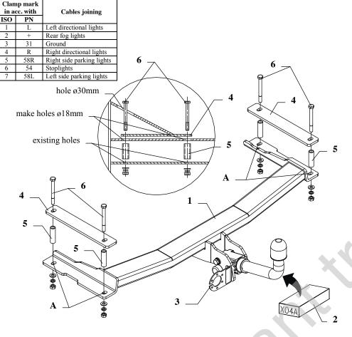
This towbar is designed to assembly in following cars: **DAEWOO ESPERO**, **4 doors**, produced since 02.1995 till 06.1997, catalogue no. **X04A** i and is prepared to tow trailers max total weight **1200 kg** and max vertical load **70 kg**.
