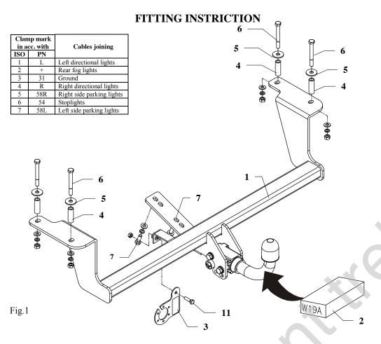
This towing hitch is designed to assembly in following car: **SUZUKI IGNIS II, 3/5 doors, 2/4WD** produced since 09.2003 till 2008 (in Hungary), catalogue no. **W19A** and is prepared to tow trailers max total weight **800** kg and max vertical load **50** kg.
