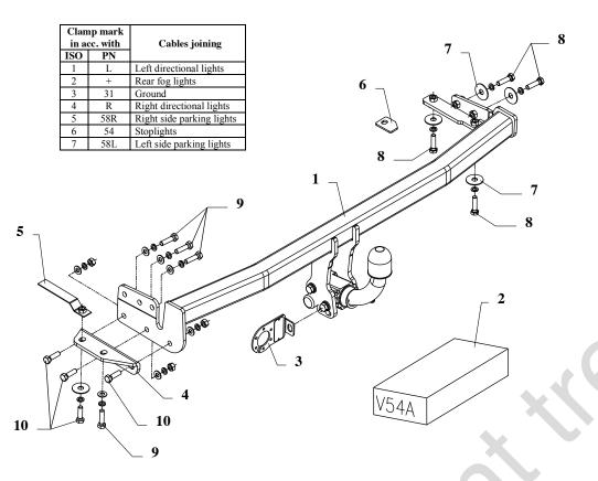
This towbar is designed to assembly in following cars: **NISSAN PRIMERA 4/5 doors**, (**P11**), produced since 09.1996 till 08.1999, catalogue no. **V54A** and is prepared to tow trailers max total weight **1700 kg** and max vertical load **75 kg**.
