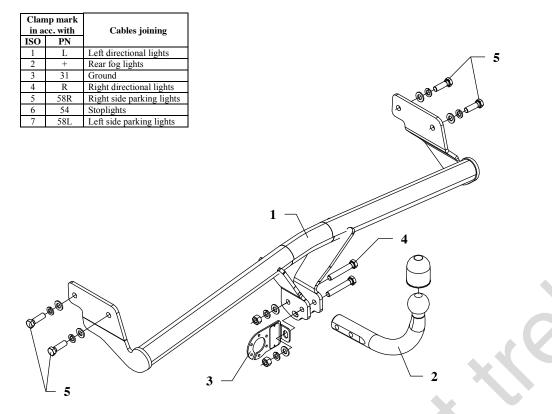
This towbar is designed to assembly in following cars: **KIA RIO II, 5 doors,** produced since 08.2005 till 09.2009, catalogue no. **T50** and is prepared to tow trailers max total weight **1100 kg** and max vertical load **50 kg**.
