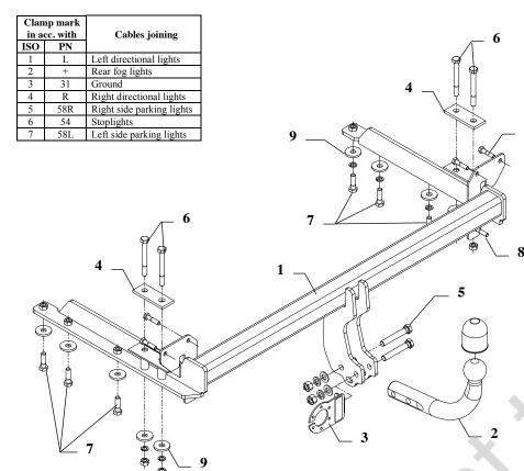
This towbar is designed to assembly in following cars: **KIA SEPHIA II, 4 doors, KIA SHUMA II 5 doors (FB),** produced since 10.1997 till 12.2004, catalogue no. **T06** and is prepared to tow trailers max total weight **1350 kg** and max vertical load **50 kg**.
