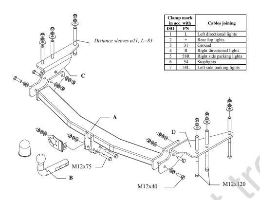
This towbar is designed to assembly in following cars: **SSANG YONG REXTON** produced since 04.2002 till 06.2006, catalogue no. **SY01** and is prepared to tow trailers max total weight **3500 kg** and max vertical load **140 kg**.
