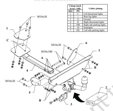
This towbar is designed to assembly in following cars: **FIAT PUNTO**, 3/5 door (176), produced since 09.1993 till 08.1999, catalogue no. **R07A** and is prepared to tow trailers max total weight 1300 kg and max vertical load 50 kg.
