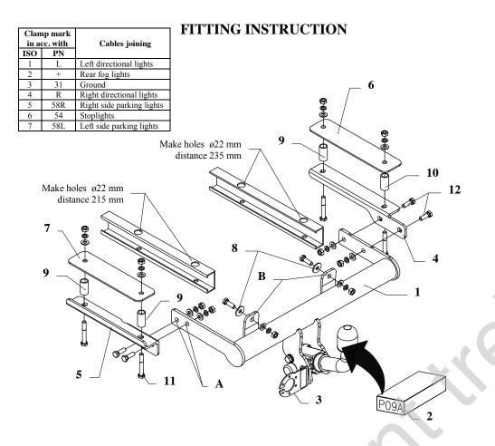
This towbar is designed to assembly in following car: CITROEN SAXO 3/5 doors, produced since 05.1996 till 09.2003, catalogue no. P09A and is prepared to tow trailers max total weight 1100 kg and max vertical load 50 kg.
