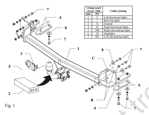
This towbar is designed to assembly in following car: MAZDA PREMACY 5 doors, VAN produced since 11.1999 till 06.2005, catalogue no. M43A and is prepared to tow trailers max total weight 1600 kg and max vertical load 50 kg.
