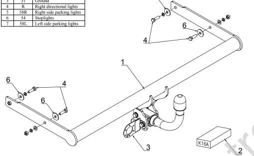
This towing hitch is designed to assembly in following cars: **VOLKSWAGEN GOLF III VARIANT, ESTATE, 4x4,** produced since 10.1993 till 07.1999, catalogue number **K16A** and is prepared to tow trailers max total weight **1500 kg** and max vertical load **75 kg**.
