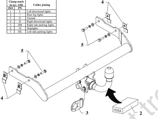
This towbar is designed to assembly in following car: SKODA FELICIA ESTATE, produced since 07.1995 till 06.2001, catalogue no. H06A and is prepared to tow trailers max total weight 1200 kg and max vertical load 50 kg.
