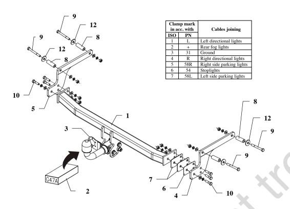
This towbar is designed to assembly in following car: **DACIA LOGAN I, 4 doors,** produced since 09.2004 till 06.2008 and since 07.2008 till 12.2012, catalogue number **G47A** and is prepared to tow trailers max total weight **1100 kg** and max vertical load **75 kg**.
