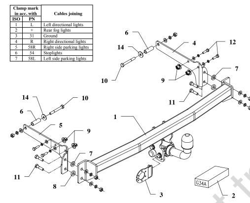
This towing hitch is designed to assembly in following cars: **RENAULT CLIO I, 3/5 doors, except 16V i 1.8 RSI,** catalogue no. **G34A**, produced since 01.1991 till 02.1998 and is prepared to tow trailers max total weight **1100 kg** and max vertical load **75 kg**.
