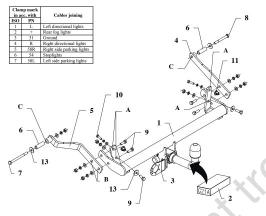
This towbar is designed to assembly in following cars: **RENAULT MEGANE I, 5 doors, except Coupe/Cabrio,** produced since 11.1995 till 02.1999, catalogue no. **G21A** and is prepared to tow trailers max total weight **1300kg** and max vertical load **65kg**.
