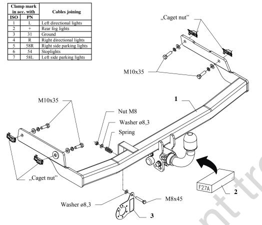
This towbar is designed to assembly in following car: **PEUGEOT 206, 3/5 doors, CC,** produced since 10.1998 till 2009 and **PEUGEOT 206+, 3/5 doors** produced since 2009, catalogue number **F27A** and is prepared to tow trailers max total weight **1100 kg** and max vertical load **50 kg**.
