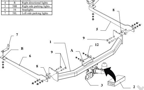
This towbar is designed to assembly in following car: **PEUGEOT 306 4 doors, except Cabrio,** produced since 10.1994 till 05.2001, catalogue number **F09A** and is prepared to tow trailers max total weight **1400 kg** and max vertical load **52 kg**.
