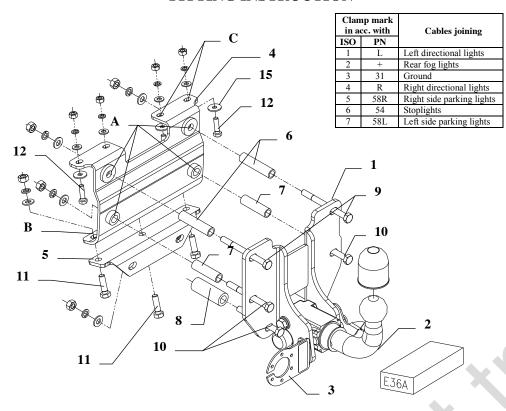
This towbar is designed to assembly in following cars: **OPEL ASTRA F ESTATE**, produced since 09.1991 till 2002, catalogue no. **E36A** and is prepared to tow trailers max total weight **1500 kg** and max vertical load **50 kg**.
