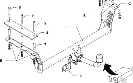
This towing hitch is designed to assembly in following cars: **OPEL OMEGA "A" CARAVAN, ESTATE,** produced since 09.1986 till 03.1994, catalogue no. **E15A** and is prepared to tow trailers max total weight **2000 kg** and max vertical load **75 kg**.
