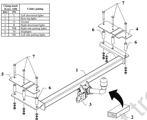
This towing hitch is designed to assembly in following cars: **OPEL ASTRA (F), 4 doors**, produced since 09.1991 till 2002, catalogue no. **E08A** and is prepared to tow trailers max total weight **1500 kg** and max vertical load **75 kg**.
