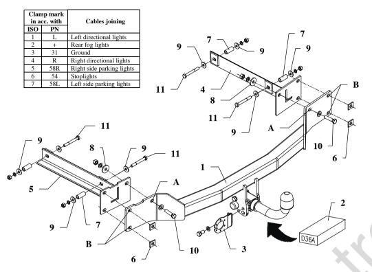
This towing hitch is designed to assembly in following cars: **MERCEDES S-CLASS (W220), except AMG,** produced since 10.1998 till 09.2005, catalogue no. **D36A** and is prepared to tow trailers max total weight **2100 kg** and max vertical load **85 kg**.
