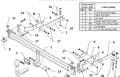
This towbar is designed to assembly in following cars: **MERCEDES 190, 4 doors (W201),** produced since 10.1988 till 08.1993, catalogue no. **D04** and is prepared to tow trailers max total weight **1500 kg** and max vertical load **75 kg**.
