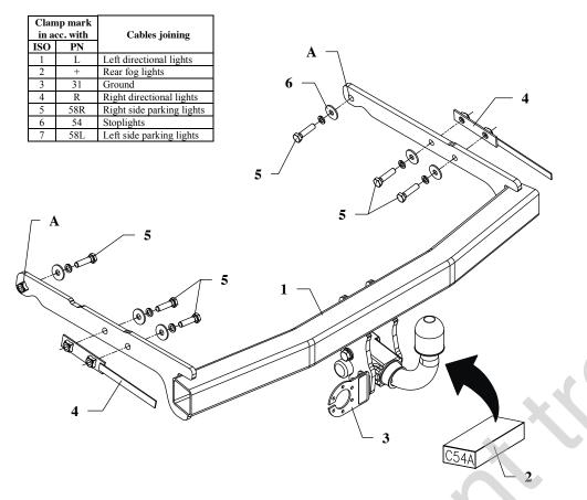
This towing hitch is designed to assembly in following car: **FORD MONDEO, 5 door (Mk4),** produced since 05.2007 till 09.2014, catalogue no. **C54A** and is prepared to tow trailers max total weight **2120** kg and max vertical mass **80 kg**.
