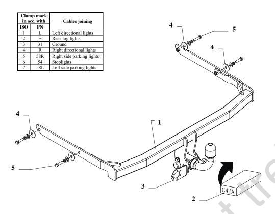
This towbar is designed to assembly in following car: **FORD FUSION, 5 doors, VAN,** produced since 09.2002 till 09.2005 and since 10.2005, catalogue no. **C43A** and is prepared to tow trailers max total weight **900 kg** and max vertical load **50 kg**.
