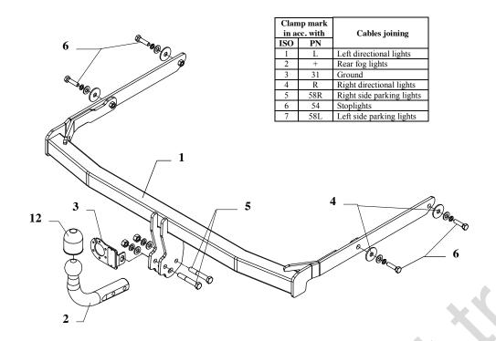
This towing hitch is designed to assembly in following car: **FORD FUSION, 5 doors, VAN,** produced since 09.2002 till 09.2005 and since 10.2005, catalogue no. **C43** and is prepared to tow trailers max total weight **900 kg** and max vertical load **50 kg**.
