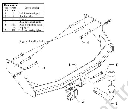
This towing hitch is designed to assembly in following cars: **FORD TRANSIT, metal build-up, also MAXI. loading platform,** produced since 11.1991 till 04.2000, catalogue no. **C18** and is prepared to tow trailers max total weight **2000 kg** and max vertical mass **75 kg**. Towbar is designed in way excluding diassemble, cut out or drill a bumper.
