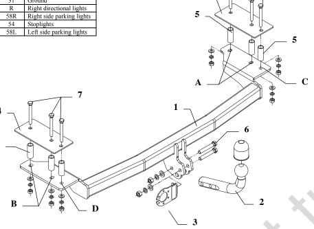
This towbar is designed to assembly in following cars: FORD ESCORT I, 3/5 doors, produced since 01.1986 till 09.1990, catalogue no. C007 and is prepared to tow trailers max total weight 1200 kg and max vertical mass 50 kg.
