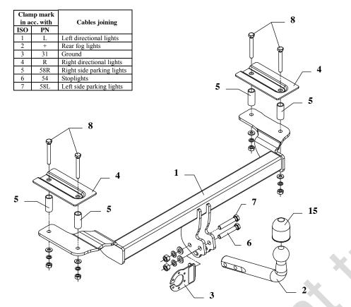
This towbar is designed to assembly in following cars: FORD FIESTA, 3/5 doors, except Sport, produced since 01.1996 till 04.2002 and MAZDA 121, 3/5 doors (JASM/JBSM), produced since 03.1996 till 08.1999, catalogue no. C002 and is prepared to tow trailers max total weight 950 kg and max vertical load 50 kg.
