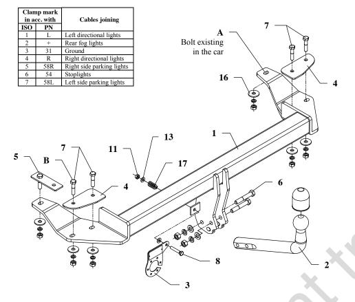
This towbar is designed to assembly in following cars: **AUDI A8, 4 door, QUATTRO (S8),** produced since 06.1994 till 09.2002, catalogue no. **A17** and is prepared to tow trailers max total weight **2350 kg** and max vertical load **75 kg**.
