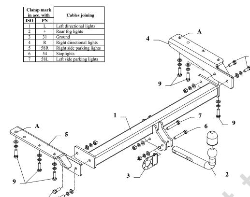
This towbar is designed to assembly in following cars: **TOYOTA LANDCRUISER**, **3 door J90/J95**, produced since 04.1996 till 12.2002, catalogue no. **O45** and is prepared to tow trailers max total weight **3500 kg** and max vertical load **140 kg**.
