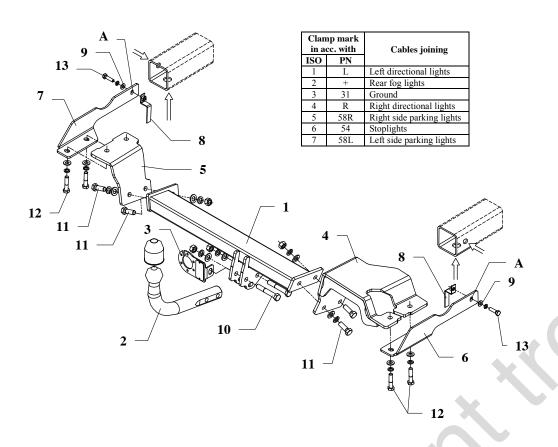
This towing hitch is designed to assembly in following cars: **TOYOTA YARIS, 3/5 doors, (CP10), Japanese and French version except TS,** produced since 04.1999 till 12.2005, catalogue no. **O24** and is prepared to tow trailers max total weight **900 kg** and max vertical load **50 kg**.
