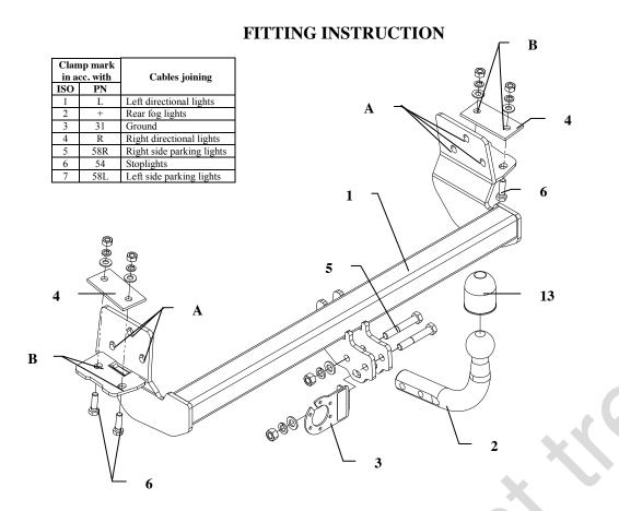
This towbar is designed to assembly in following cars: **TOYOTA COROLLA Station Wagon ESTATE (E11)** produced since 06.1997 till 12.2001, catalogue no. **O17** and is prepared to tow trailers max total weight **1400 kg** and max vertical load **75 kg**.
